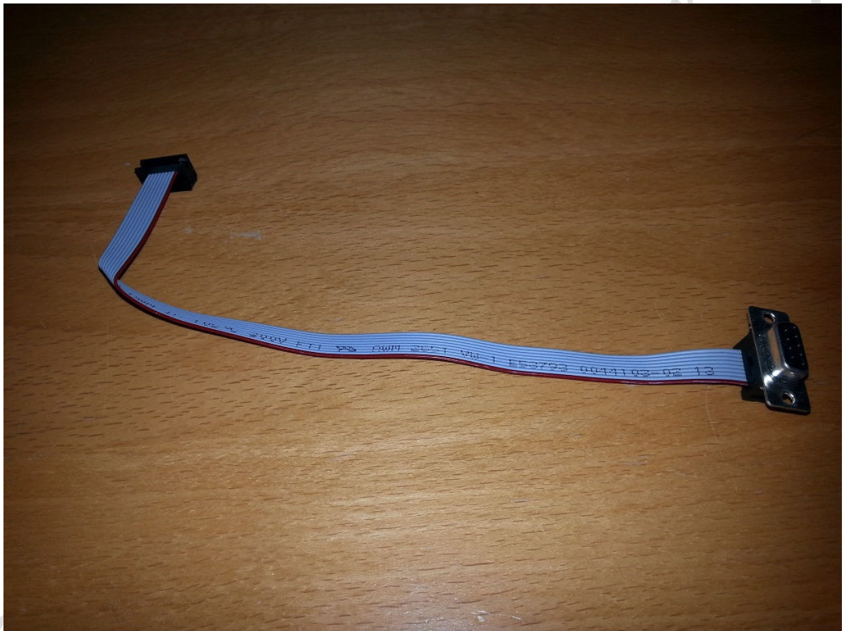
Figure 2: Completed serial port cable assembly
